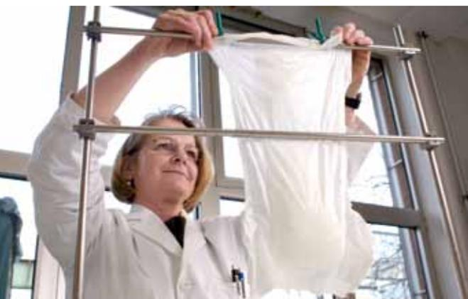
A stopwatch is used to measure the speed with which the diaper absorbs liquid. Just one of many tests our scientists perform to make superabsorbents even more efficient and effective.
